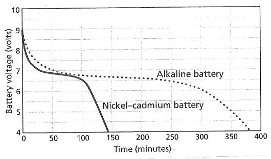
The transparency shows how the voltage of two batteries changes when they are used to power the same kind of electrical device.
